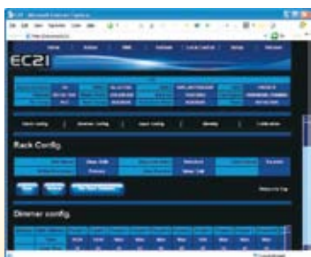
EC21 configuration and status reporting is accessible from any wired or wireless network PC or PDA and networked Strand consoles via Web browser.
